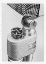
Increases in bass response, which occur mostly when microphones are used for close talking purposes, can be compensated by employing the bass cut switch to attenuate the low frequencies by 7 or 12 db (at 50 cycles). The position —12 db should, however, only be employed when the microphone is used at very short speaking distances.
